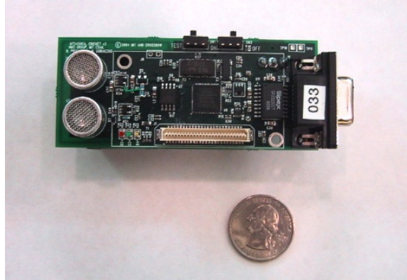
Figure 2-4: A photo of the version 2 Cricket, which can function as a listener or a beacon.
