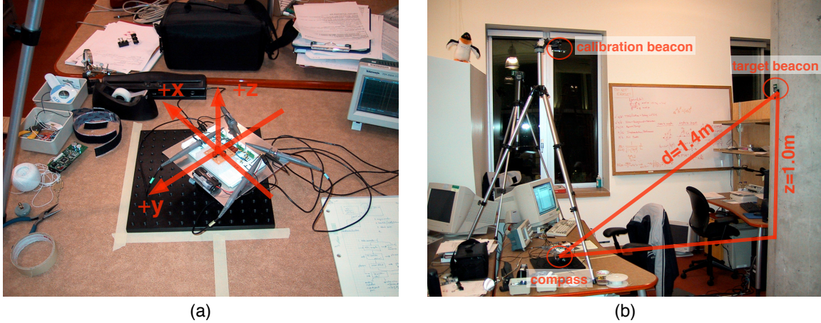
Figure 5-1: Photos of the beacon localization experiment. (a) shows the Compass prototype mounted on the rotating platform with an overlay of the axes in the Compass' coordinate space. (b) shows the lab space with the positions of the calibration beacon, target beacon, and Compass.
