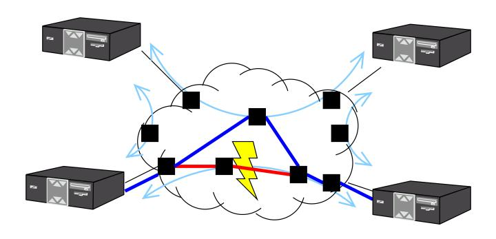
Any-to-any communication transparently routing around failures
